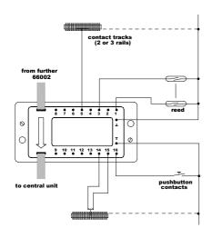
The feedback signal can come from contact tracks, reed contact, pushbuttons, track occupation detectors (ex. MO 66100) or other modules.
